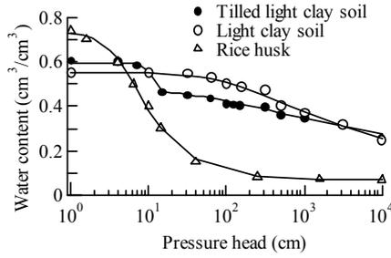
Fig. 2. Soil water retention curves of materials.
