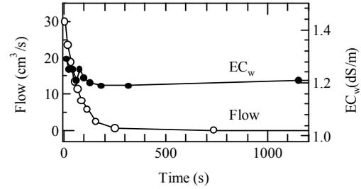
Fig. 3. Change of drainage rate from soil tank.
