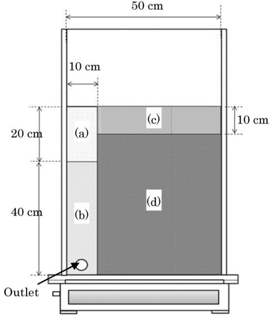
**Fig. 1. Schematic diagram of the soil tank, (a) filled soil zone (FZ), (b) rice husk zone (RHZ), (c) plow zone (PZ), (d) no-tilled zone (NTZ).**
