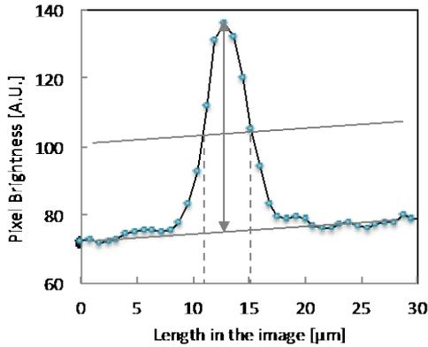
(b) Brightness profile of the latex bead image. The full width at half maximum was measured as about 4  $\mu\text{m}$ .
