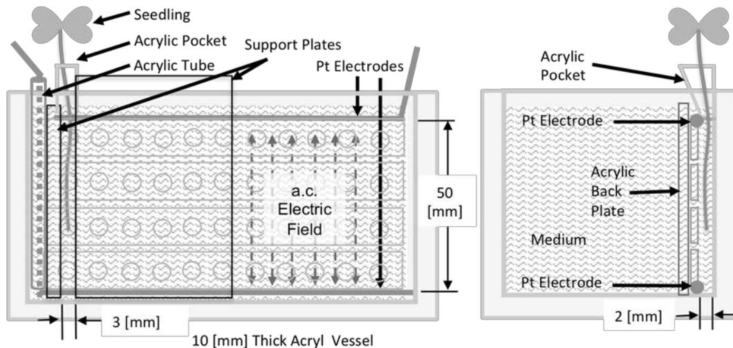
**Fig. 1. The schematic of the culture vessel for electric field application in solution.** Culture vessel is made by 10 mm thick acrylic resin plate. 2 mm gap of front compartment is separated by perforated back plate from bulk medium. Pt electrodes are installed on top and bottom of the front compartment. Plant seedling was placed in a acrylic pocket on top of the front compartment. The plant root is let to grow through a bottom hole of the pocket into the front compartment.
