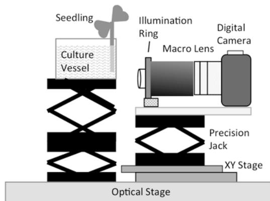
**Fig. 3. Schematic of the Magnified time lapse image capture system.**
