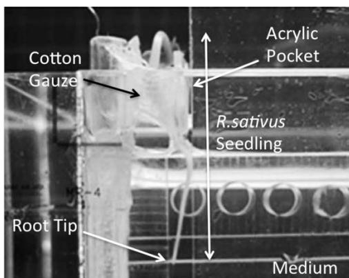
**Fig. 2. *R. sativus* seedling in the water culture vessel.** A seedling was placed in the acryl pocket on top of the culture vessel. The growing root tip of the seedling can be seen through transparent acrylic window. The root go down through a hole at the bottom of the pocket and grow along the narrow channel.
