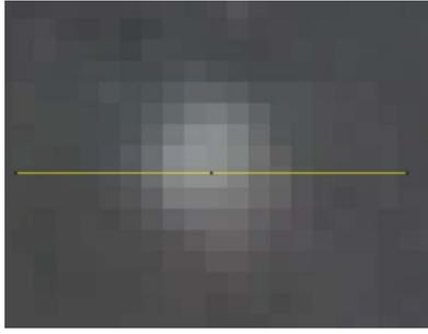
(a) Optical image of latex bead, captured by the lens system. Brightness of the image was measured along the horizontal line.
