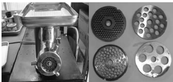
Fig. 1. Mincing machine with 4 sizes of plate.
