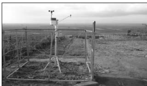
Fig. 1. Automatic meteorological observation system in the command area.
