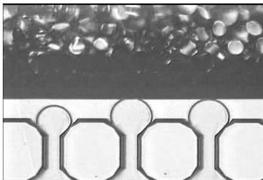
**Fig. 4.** Microscopic image of emulsification behavior from a grooved MC; regular droplet generation at low dispersed phase flux.
