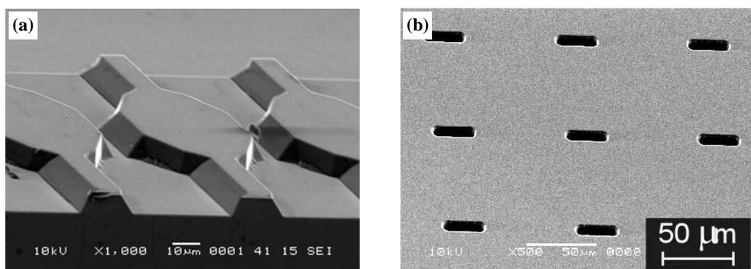
**Fig. 1.** Scanning electron microscopy (SEM) images of silicon arrays of microchannels: (a) grooved MC; (b) oblong straight-through MC.
