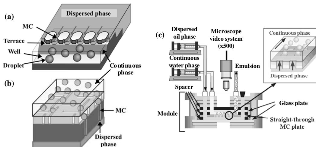
Fig. 2. Schematic illustration of droplet generation: (a) grooved MC; (b) asymmetric straight-through MC; (c) typical experimental setup image for straight-through MC emulsification.
