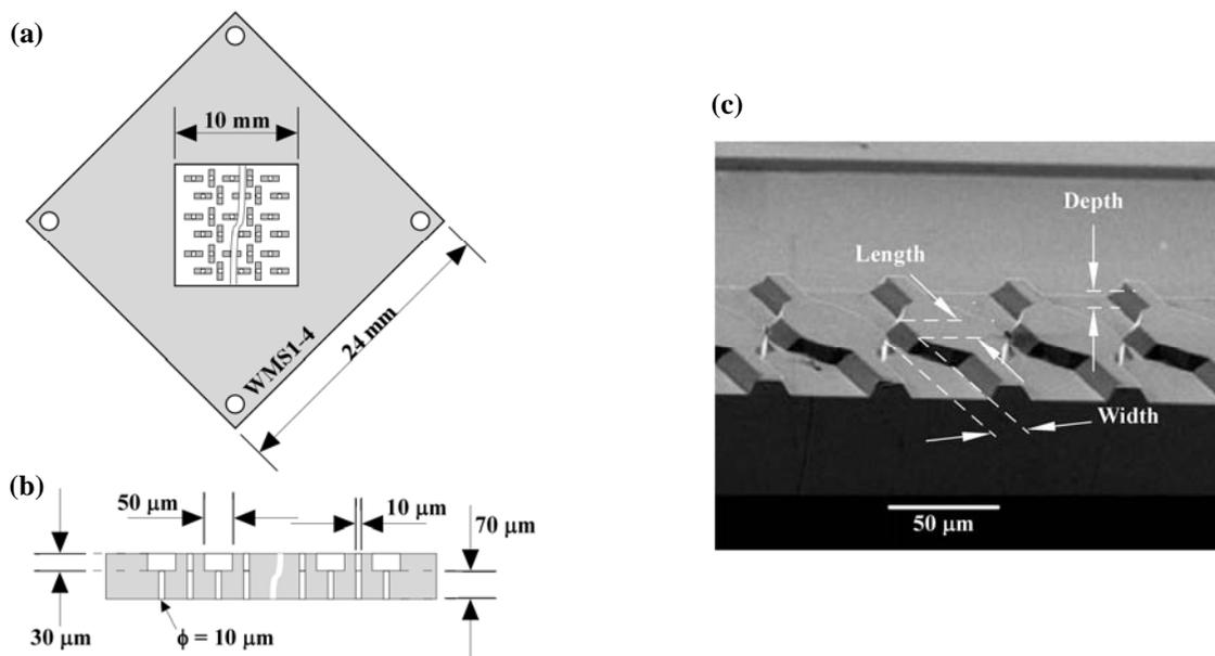
Fig. 3. Schematic illustration of MC: (a) Top view of alternate horizontal-vertical asymmetric straight-through MC plate WMS 1-4; (b) Cross-sectional view of MC WMS 1-4; (c) SEM micrograph of grooved MC plate MS 308, depicting its dimensions.
