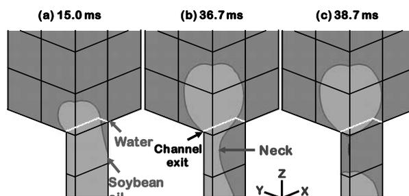
**Fig. 5.** Emulsification behavior using straight-through MC, calculated by computational fluid dynamics. Successful formulation of a droplet with a diameter of about  $35 \mu\text{m}$  from an elliptic straight-through MC (longer line,  $40 \mu\text{m}$ ; shorter line,  $10 \mu\text{m}$ ).
