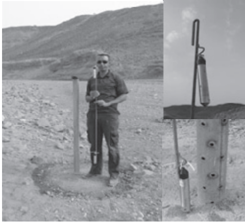
Fig. 4. Water- level pressure sensor installed in perforated steel pipe for protection in the watershed of Kourtimalei reservoir.
