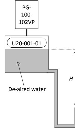
**Fig. 1. Schematic diagram of the experiment to verify the accuracy of the water level logger (U20-001-01) by comparison with PG-100-102VP.**
