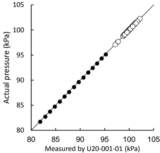
**Fig. 2.** Comparison of the atmospheric pressures between data measured by U20-001-01 and actual data measured by PTB210 (open) and PG-100-102VP (closed).  $r^2$  and RMSE are coefficient determination and root mean square error, respectively.
