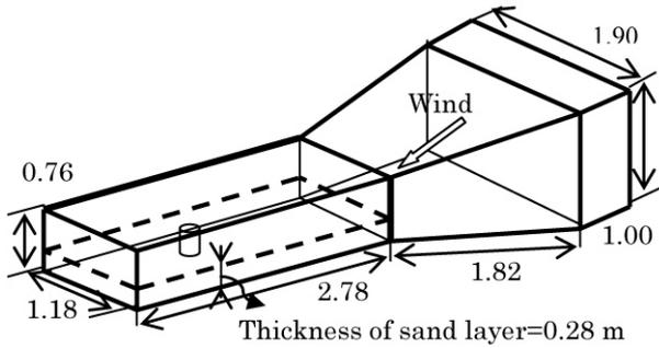
Fig.1. Configuration of experimental apparatus.
