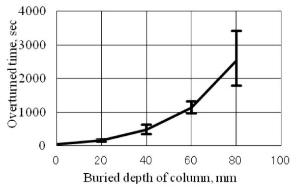
Fig. 4. Buried depth and overturned time.
