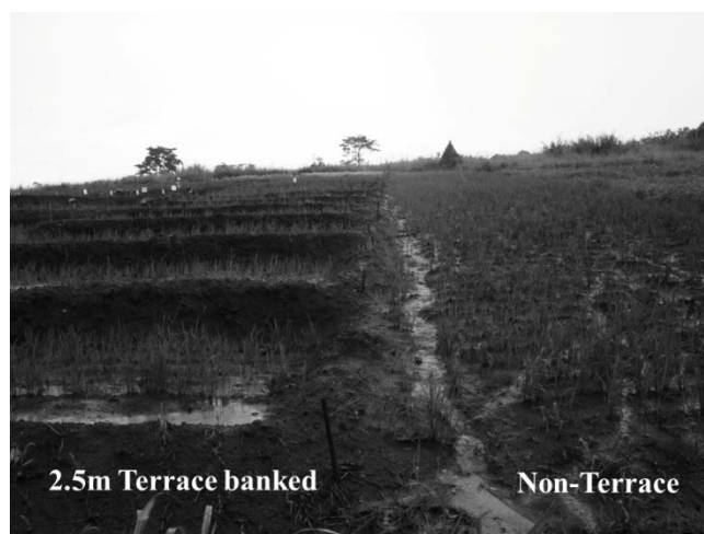
Fig. 3. 2.5m-Terrace banked with soil (left) and control (right) during a downpour. Terraces retain rainfall but water escapes down the control field.
